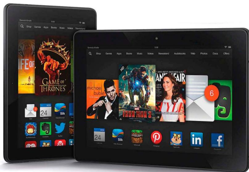
**DOTTY DISPLAYS:** The Kindle Fire HDX is one of the first consumer devices to use displays with quantum dots.
