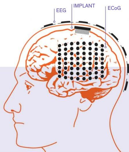
**THREE WAYS TO TAP THE BRAIN** To record the activity of brain cells, neuroscientists can use implanted electrodes that penetrate the cortex. This method provides the clearest signal, but it's also the riskiest. In contrast, scalp electrodes for electroencephalography (EEG) carry no risks, but the signal they capture is indistinct. Electrocorticography (ECoG), which uses electrodes draped over the surface of the cortex, may represent the "sweet spot," a compromise between risk and clarity.
