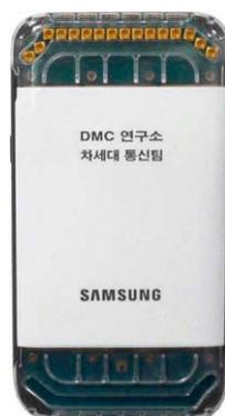
**PACKING IN PATCHES:** Samsung engineers are working to fit arrays of 28-gigahertz patch antennas into phones like the Galaxy Note II, pictured above.
